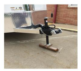
Rear Support Jacks – These are attached to the bottom of the trailer and are located at the rear. There is one on both sides of the trailer to ensure stabilization and make it safe for use/entry. To lower the rear support jacks, push them inward and pull them down to the ground. They must be set so they are firmly planted on the ground. See picture below for reference:
